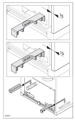
■ The covers for the brackets are designed for 16 mm and 19 mm thick carcase sides. Turn the covers so that they are in the appropriate position and fit them onto the brackets.
